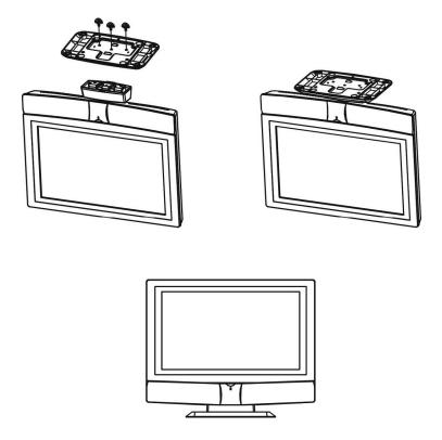
Note: L15X421 does not need the screws to install.
